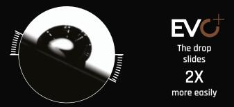
Laboratory measurements made by Drop Shape Analyzer DSA30 according to ASTM D7334-08. Angle formed by a drop of water deposited on a surface.
